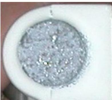
Erosion, Cavitations -- Removal of die steel and subsequent deformation of the casting.
